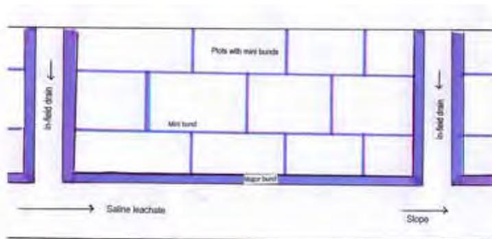
Fig 6.2 Field Drains Cross Section
